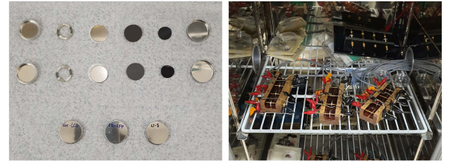
(a) Fabricated coin-cell batteries. (b) Battery testing equipment.
