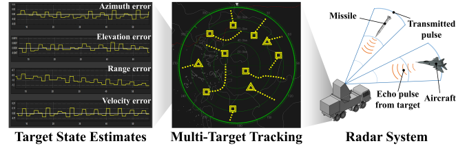
Fig. 1: The operational concept of an STR system.
